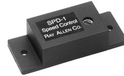
Install the speed control at any convenient location preferably near the trim switch. Secure to the airframe with two screws or simply tie onto a wire bundle using nylon straps, etc. It is not necessary to ground the case of this unit.
