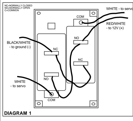
What the REL-2 Relay Deck needs from the RS2 Rocker Switch (or any switch for that matter), is a ground input on either the orange or green wires to activate the small relays inside.
